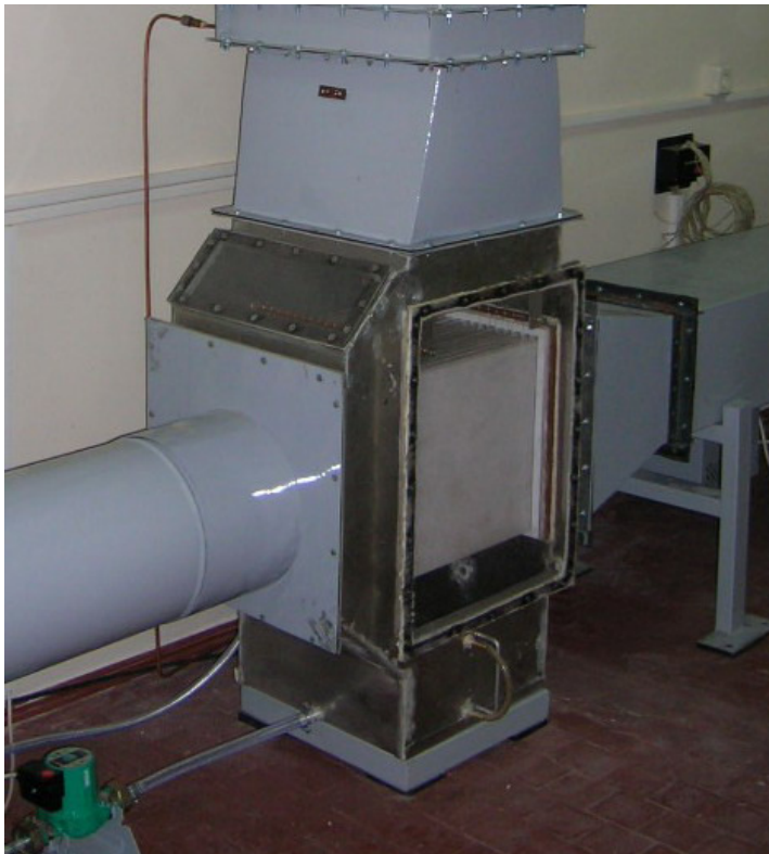
Fig. 1. Schematic diagram and photograph of the test rig to study the cross-flow heat and mass transfer devices for direct and indirect evaporative cooling of water and air. 1 – electric heater; 2 – ventilator; 3 – working chamber; 4 – liquid distributor; 5 – spray separator; 6 – air flow meter; 7 – return line; 8, 9 – air flow regulator; 10 – water flow meters; 11 – sectional meter of liquid flow rate; 12 – water tank; 13 – water pump; 14 – filter; 15 – water heater; 16 – water temperature regulator; 17, 18 – mercury thermometer and RTD sensor; 19 – pressure gauge; 20 – tank for the measurement of liquid retention; 21 – scale bar; 22 – control box.
