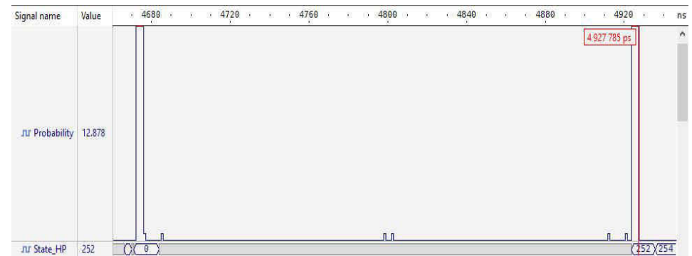
Figure 17: Upper register states that are perceived at the input of QFT and correlated with the function y = a^x \text{ mod } M , homogeneous quantum coprocessor
