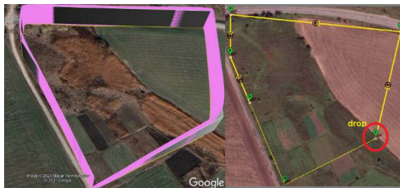
Figure 14: Copter flight trajectories according to the program (right) and obtained experimentally (left)
