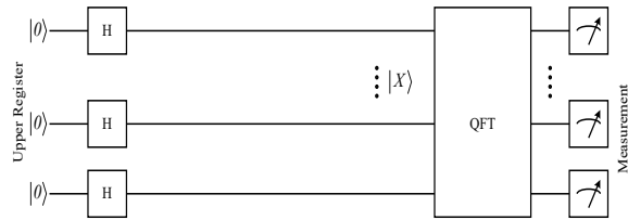
Figure 8: White noise |X\rangle generated by a quantum circuit
