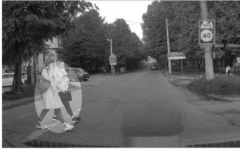
Figure 12: Resulting image with highlighted pedestrians and detected traffic sign
