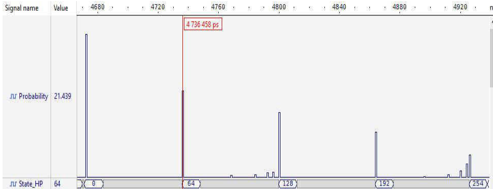
Figure 19: The number of states repetitions when determining the period of a function, homogeneous quantum coprocessor
