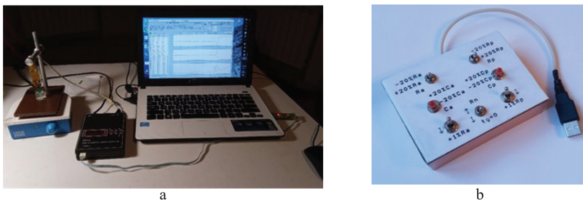
Figure 4. Photo of the hardware-software complex for the conductometric analyzer and the electrical equivalent of the differential conductometric cell.
