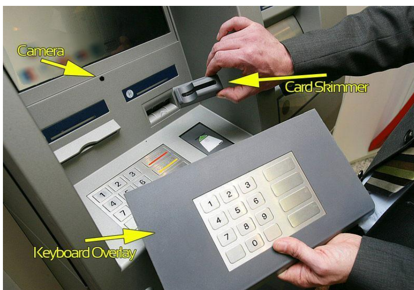
Fig. 1. Equipment for scimming, installed in the payment terminal
